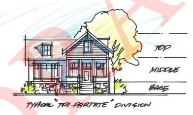
Figure 4: Definition: tripartite division in architecture is a design approach that separates a building's façade into three horizontal sections: the base, the middle, and the top.
