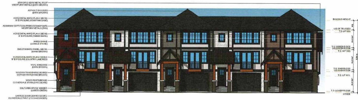
WEST ELEVATION - FRONT 1/8" = 1'-0"
