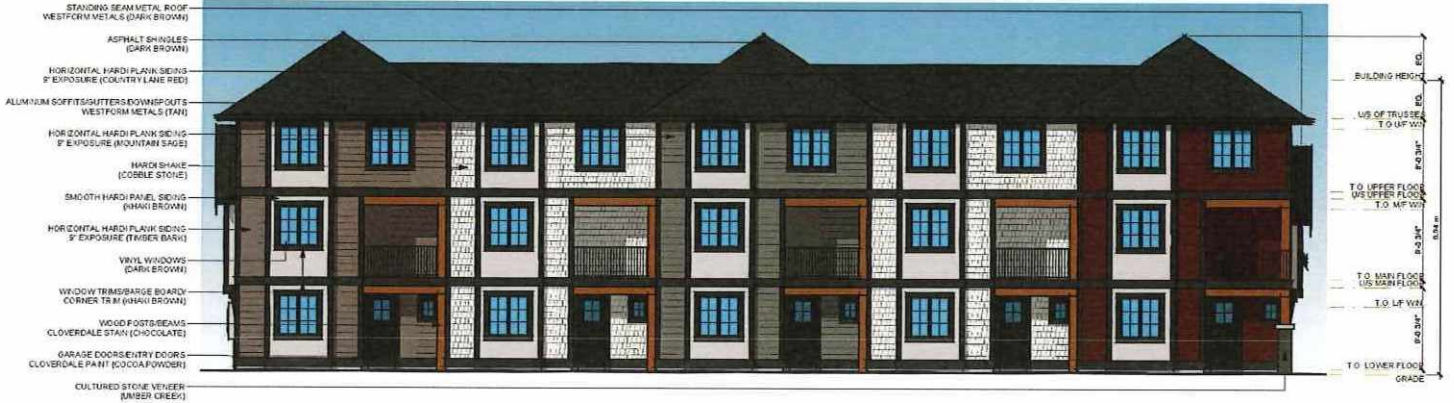
EAST ELEVATION - REAR 1/8" = 1'-0"
