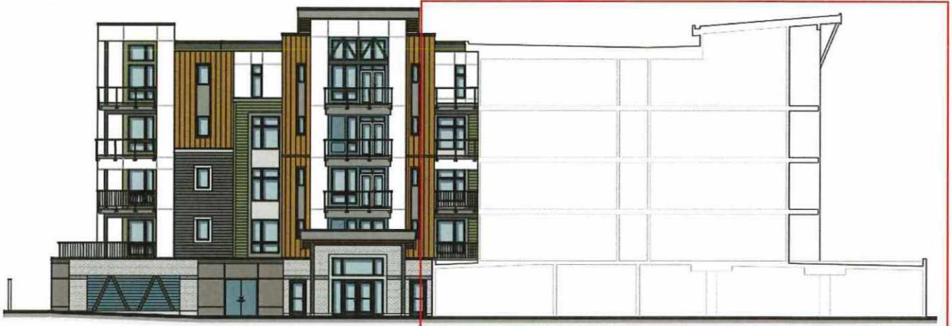
3 WOODBINE STREETScape A5.1 EXTERIOR MATERIALS - PAVED DRIVE, PAVED PAVIL, PAVED TRUNK, PERI-FRONTED METAL CLADDING (UP OF WALLS, GLASS AND FLOOR) BRASS, PAINTED CONCRETE.
